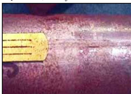
Defect in electric seam weld of 1.75-in. steel tbg, AC magnetic flux from yoke
